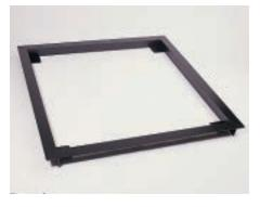
**Pit Frame w/ Pit Kit** Allows easier pit installation of 6600 base. Pit frame doubles as form for pouring concrete. Available in painted mild steel or stainless steel construction.
